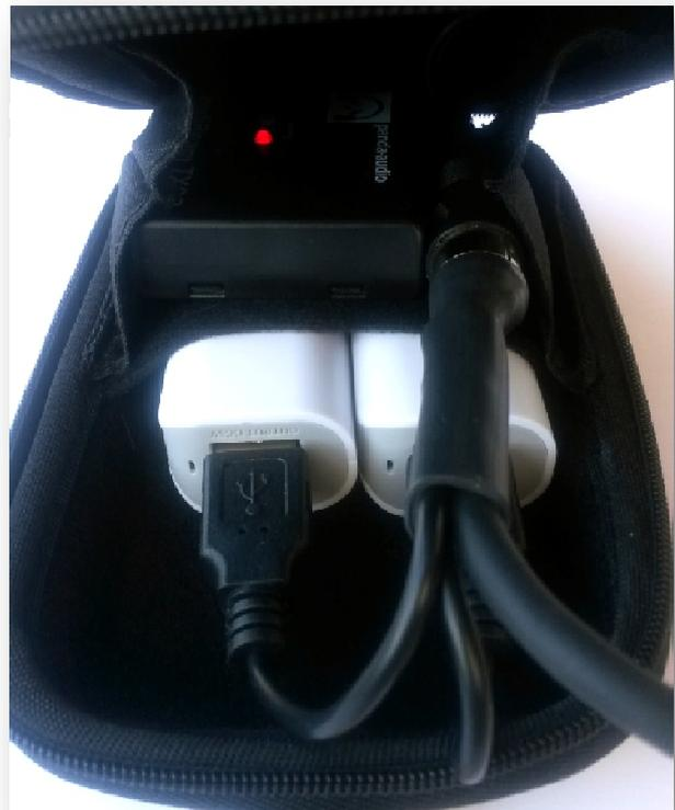
Finally, close the box by pulling up the zippers from the left and right sides. Close the body pack by carefully pushing both USB cables inside the rim of the box. Only the Midi cable leads to the outside from the top center of the belt pack.
