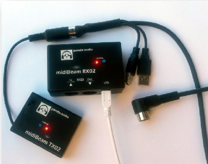
Connect the receiver with the USB mini cable to your computer. The receiver RX-02 works without a driver software, i.e. it is a true « plug-and-play » device for both Windows and MAC operating systems.
