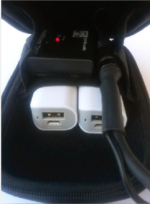
Now plug both USB connectors into the powerbanks as shown below. It is not critical, which USB plug goes to the left and right powerbank. Switch on the transmitter and check its LED status. It should stay ON constantly. If it is blinking, either the receiver RX-02 is not yet turned on, or you need to pair them manually, i.e. push the button on either of the units to synchronise them. A steady lit LED shows that a wireless connection has been established.
