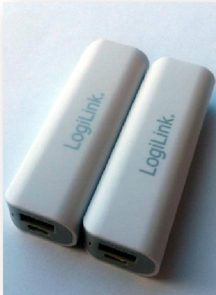
Two high-power USB power banks provide power to the Synthophone. A fully recharged set of these special accumulator batteries holds approximately 3 hours of performance time.
