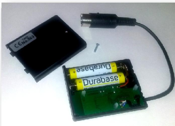
The transmitter runs on two regular AAA batteries. With a small Philips screwdriver, unlock the small screw of the the battery compartment, remove the cover and replace the batteries as shown in the picture. Please observe the correct polarity as shown. Close the cover and put the screw back in place.
